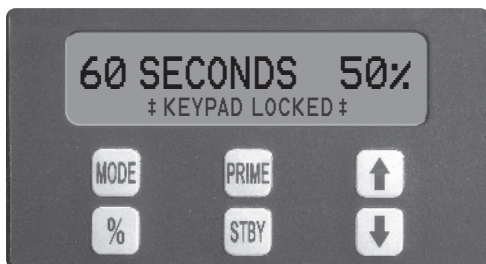
Example of control panel with keypad locked.
